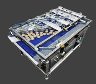
The AutoLaner is a series of controlled lanes that automatically divide a randomly distributed product stream equally into multiple lanes (typically 4 or 6). The AutoLaner is designed to be installed downstream from an MT-Series 100% Inspection System.
