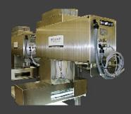
The FocalPoint<sup>™</sup> system may be positioned in various locations over a production line. It can be configured to capture product attributes such as true color, height, diameter, symmetry, length, width, and volume. Data is stored in a relational database for historic reporting and trending.
