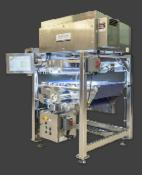
The MT-Series of systems use a highspeed, non-contact imaging method to continuously quantify a wide range of object characteristics such as top and bottom color, topping coverage, height, diameter, slope, symmetry, length and width. Results are displayed in real-time on an attached monitor and ethernet connected PC.
