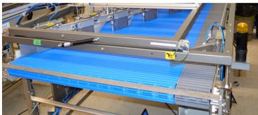
Products enter the AutoLaner randomly and are spread across the laning conveyor in a random pattern. A series of automatic product gates move products to each lane without jamming. Once inside the lanes, the flow of each lane is metered so that a precise number of objects is fed to downstream equipment (typically the slicer). Metering the outflow of individual pieces is performed using a combination of sensors and a high-speed controller to dynamically control the gates.
