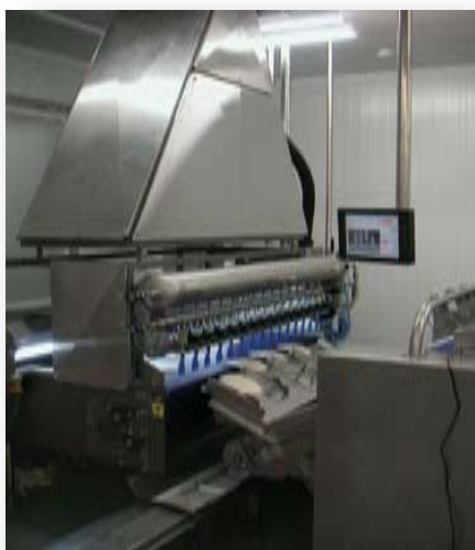
The Dipix T60/In-Line Tortilla Inspection System
